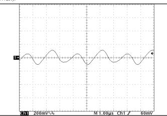
**Figure 10:** Output voltage ripple, Vout, at nominal input voltage and rated load current (200 mV/div). Load capacitance:  $1\mu F$  ceramic capacitor and  $15\mu F$  tantalum capacitor. Bandwidth: 10 MHz. See Figure 17.
