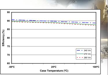
Figure 2: Efficiency at nominal output voltage and 60% rated power vs. case temperature for minimum, nominal, and maximum input voltage.
