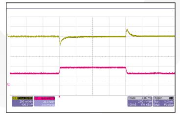
**Figure 11:** Output voltage response to step-change in load current (50%-75%-50% of lout(max);  $dI/dt = 0.1 A/\mu s$ ). Load cap: 1  $\mu$ F ceramic and 15  $\mu$ F tantalum capacitors. Ch 1: Vout (200mV/div), Ch 2: lout (20A/div).
