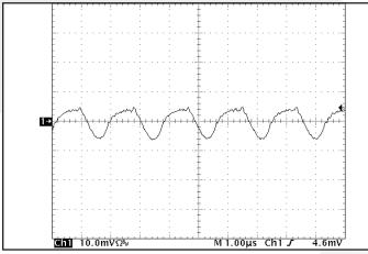
**Figure 9:** Input terminal current ripple,  $i_C$ , at full rated output current and nominal input voltage with  $100\mu$ H source impedance and  $47\mu$ F electrolytic capacitor (200 mA/div). Bandwidth: 20MHz. See Figure 17.
