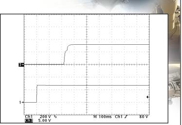
Figure 8: Turn-on transient at full resistive load and zero output capacitance initiated by Vin. ON/OFF Pin previously low. Ch 1: Vin (200V/div). Ch 3: Vout (5V/div).
