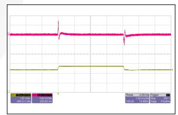
**Figure 12:** Output voltage response to step-change in input voltage (250V/ms). Load cap:  $1\mu$ F ceramic and  $15\mu$ F tantalum capacitors. Ch 1: Vin (100V/div), Ch 2: Vout (100mV/div).
