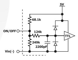
Figure B: Internal ON/OFF pin circuitry
