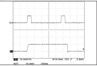
*Figure 18:* Load current (50*A*/div) as a function of time (10ms/div and 100ms/ div) when the converter attempts to turn on into a 10 m $\Omega$  short circuit.
